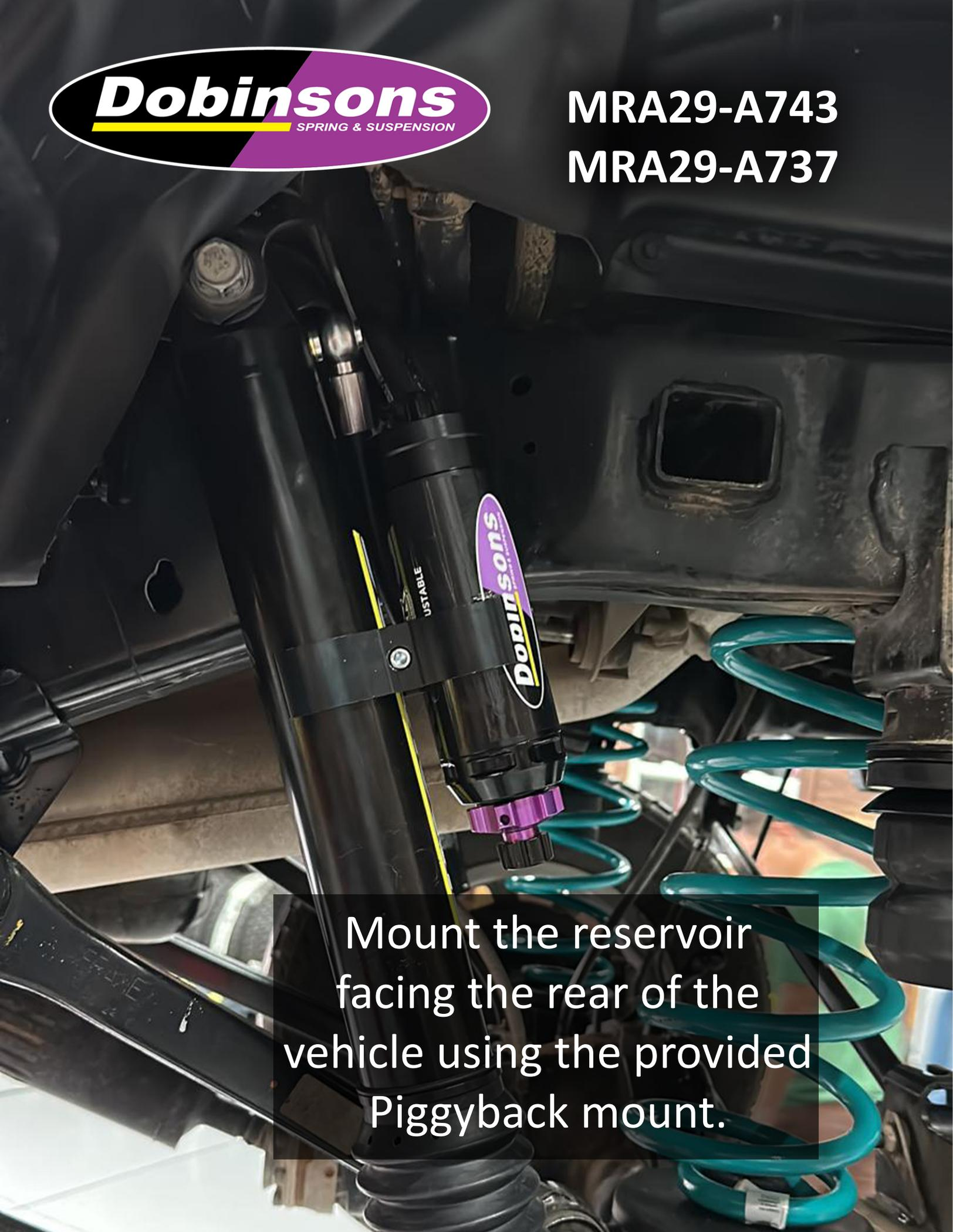
Mount the reservoir facing the rear of the vehicle using the provided Piggyback mount.
